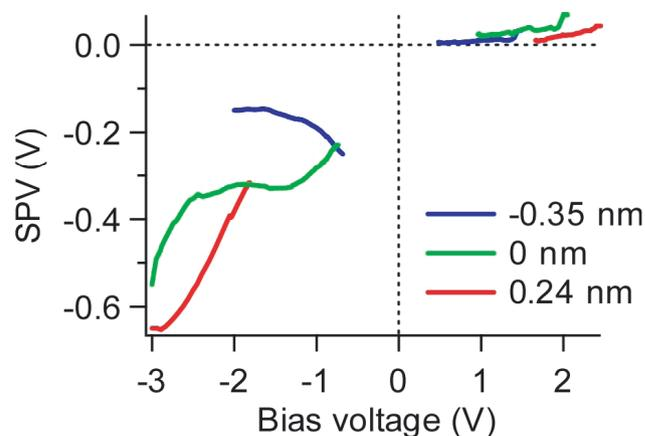
FIG. 6: Tip-sample distance dependence of SPV. The green spectrum was obtained at the position of 0 nm in Figs. 5(a), 5(c) and 5(d). Blue and green spectra were obtained at two different positions of -0.35 nm (closer) and 0.24 nm (far) from the set point. Horizontal axis represents the distance of tip retraction from the set point.
