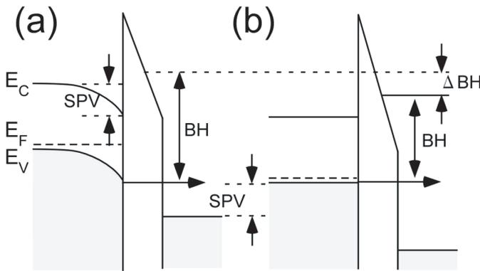
FIG. 2: Schematic illustrations of MIS structures in cases (a) without and (b) with photoillumination.
