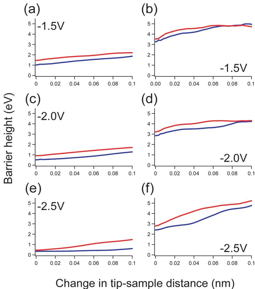
FIG. 5: Tip-sample distance and bias-voltage dependences of LBH obtained using two different tips ((a), (c) and (e) for the first tip and (b), (d) and (f) for the other) under dark (blue) and photoilluminated (red) conditions, respectively. Horizontal axis represents the distance of tip retraction from the set point.
