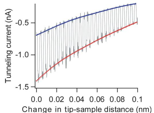
FIG. 4:  $I$ - $Z$  curve ( $Z$ : tip-sample distance) measured under chopped photoillumination. Horizontal axis represents the distance of tip retraction from the set point.
