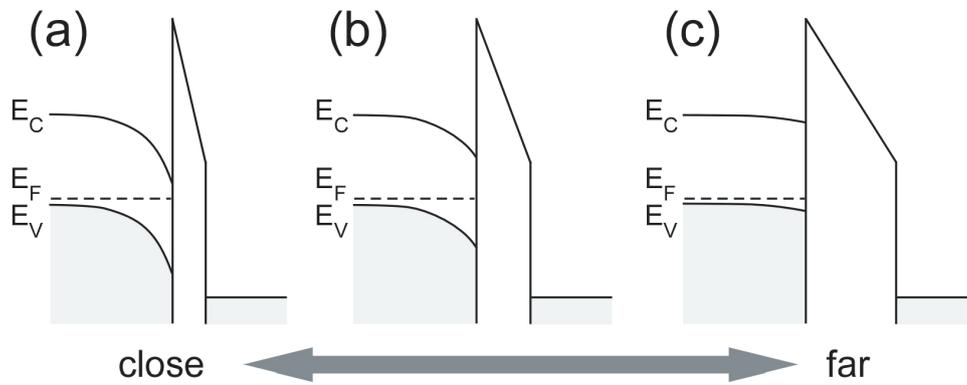
FIG. 1: Characteristics of tip-induced band bending (TIBB) depending on tip-sample distance.
