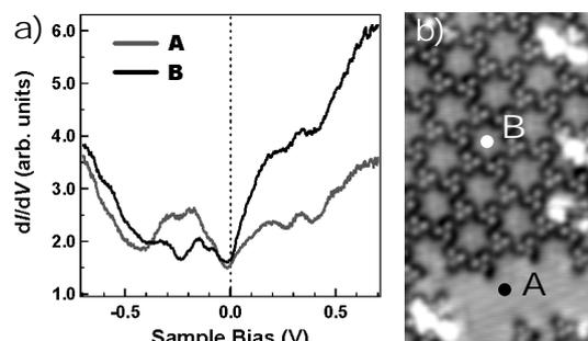
Fig. 2 (a):  $dI/dV$  measurements on Cu(111) substrate and Cu area surrounded by trimers in molecular structure indicated by A and B in the left image (b), respectively.
