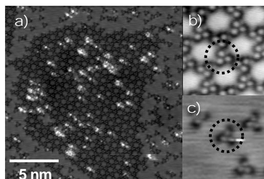
Fig. 1 STM image of glycine molecules adsorbed on Cu(111) surface ( $V_s = -0.5$  V,  $I = 1.0$  nA)
