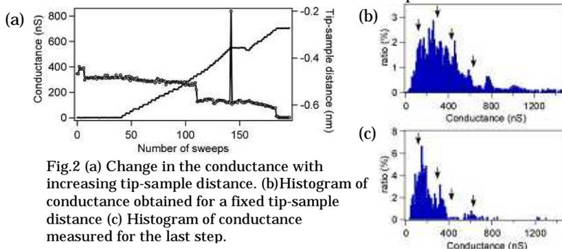
Fig.2 (a) Change in the conductance with increasing tip-sample distance. (b) Histogram of conductance obtained for a fixed tip-sample distance (c) Histogram of conductance measured for the last step.
