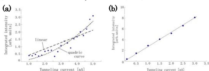
Fig. 2. Tunneling-current dependence of light intensity from the molecular films of (a) CuPc (b) ZnPc.
