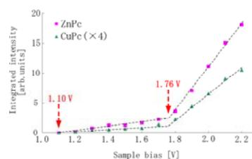
Fig. 1. Sample-bias dependence of light intensity from the molecular films (CuPc and ZnPc).
