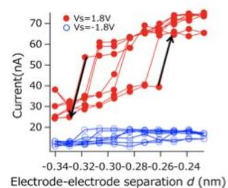
Fig.2 Conductance switching with electrode distance
