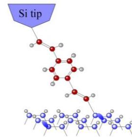
Fig.1 Formation of a Si/single molecule/Si junction.
