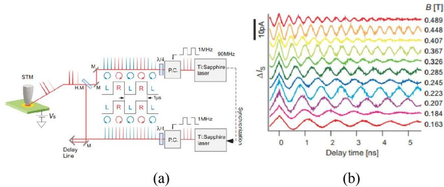
**Fig.1. (a)** The schematic of the OPP-STM. P.C is the pockels cell used to modulate the polarization states. **(b)** The magnetic field dependence of spin precessions under the OPP-STM setup, the spin precession occurs at the Larmor frequency  $\omega = g\mu_B B / \hbar$ , where  $g$  is the Landé's  $g$  factor,  $B$  is the magnetic field,  $\mu_B$  is Bohr magneton and  $\hbar$  is Dirac constant.
