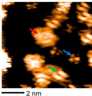
Figure 1. STM image of  $\text{Mo}_{1-x}\text{Re}_x\text{S}_2$  monolayer
