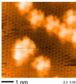
Figure 1. STM image of MoS<sub>2</sub> monolayer (V<sub>s</sub>=-2.2V)
