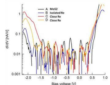
Figure 3. dI/dV spectrum measured on Re atoms and MoS<sub>2</sub>
