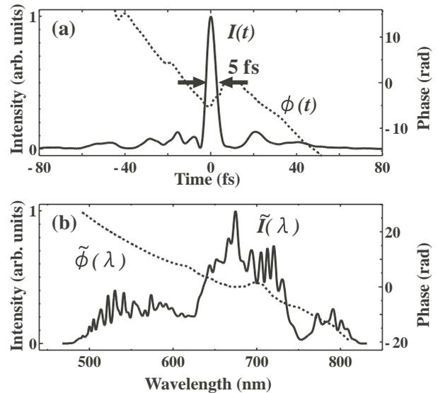
Fig. 4. (a) Retrieved pulse intensity (solid curve) and phase (dashed curve) in the time domain. (b) Retrieved spectrum (solid curve) and spectral phase (dashed curve).
