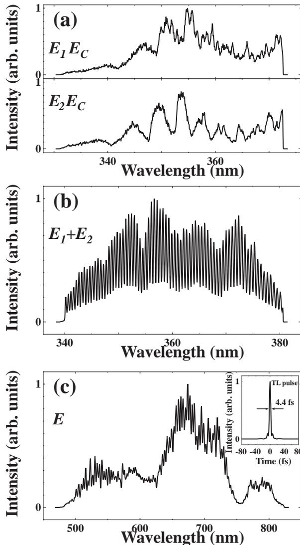
Fig. 3. (a) Two measured sum-frequency spectra,  $E_1E_C$  and  $E_2E_C$ . (b) Measured interferometric second-harmonic spectrum  $(E_1+E_2)^2$ . (c) Measured spectrum of the input pulse  $E$ , and the 4.4 fs transform-limited pulse (inset).
