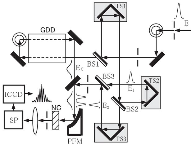
Fig. 1. SPIDER setup: BS1-BS3, beam splitters (450–1300 nm); GDD, TF5 glass block; TS1, translation stage for adjustment of temporal overlap of the short pulse pair with the stretched pulse; TS2, TS3, translation stage for adjustment of delay; PFM, aluminum 50 mm focussing parabolic mirror; NC, nonlinear crystal (25- $\mu\text{m}$ -thick type-II BBO); SP, spectrometer; ICCD, intensified charge-coupled device.
