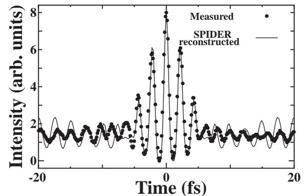
Fig. 5. Comparison of the measured interferometric autocorrelation (IAC) trace (dots) with the SPIDER-reconstructed IAC trace (solid curve).
