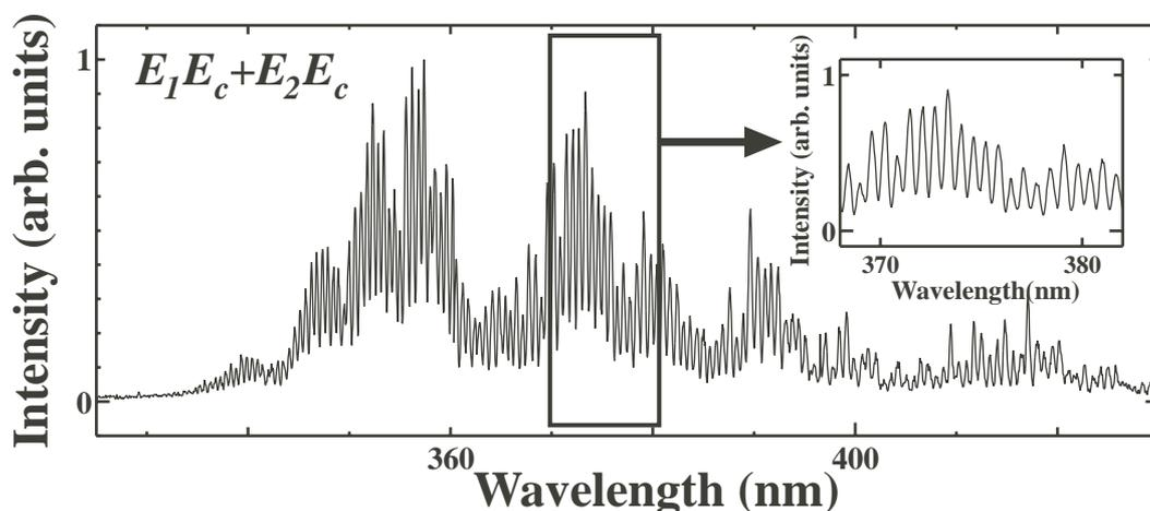
Fig. 2. Measured SPIDER interferogram signal.
