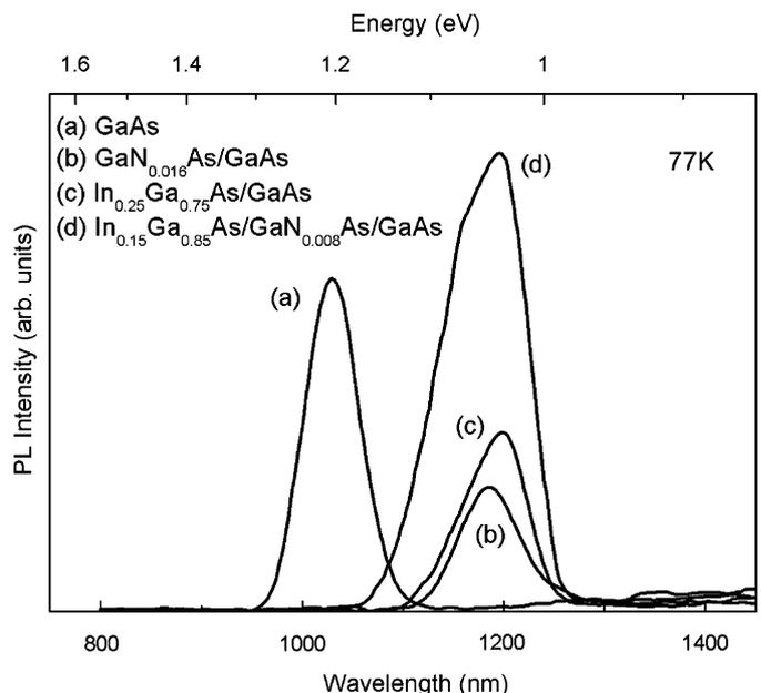
Fig. 2. PL spectra measured at 77 K for InAs QDs embedded with (a) GaAs (reference), (b)  $\text{GaN}_{0.016}\text{As}_{0.984}$  SCL, (c)  $\text{In}_{0.25}\text{Ga}_{0.75}\text{As}$  SRL, and (d)  $\text{In}_{0.15}\text{Ga}_{0.85}\text{As}/\text{GaN}_{0.008}\text{As}_{0.992}$ , respectively.
