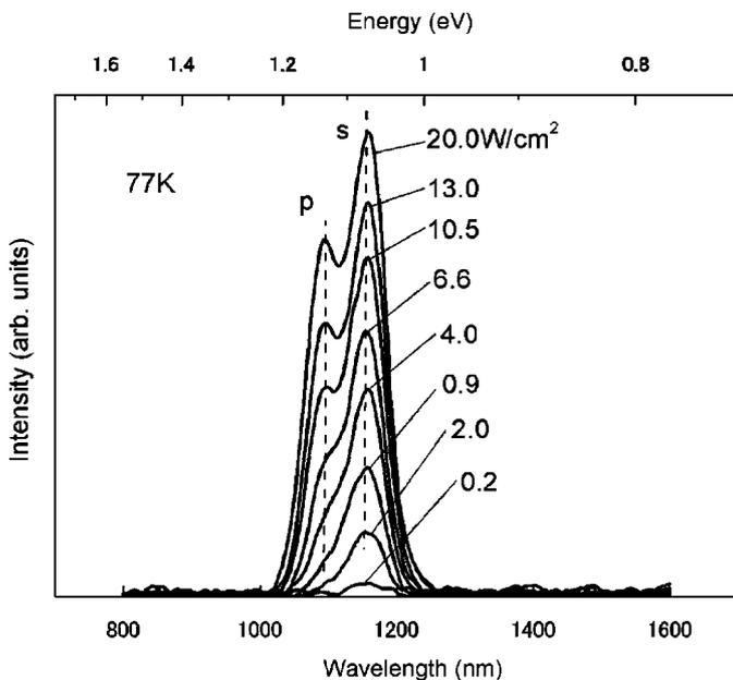
Fig. 5. Dependence of PL characteristics on excitation intensity for sample embedded with a combined set of  $\text{In}_{0.15}\text{Ga}_{0.85}\text{As}/\text{GaN}_{0.008}\text{As}_{0.992}$  layers. The excitation intensity was varied from 0.2 to  $20.0 \text{ W/cm}^2$ . S-peak indicates an emission from the ground state, while p-peak shows that from the first excited state of QDs, respectively.
