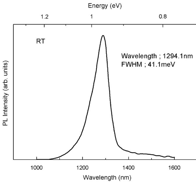
Fig. 3. PL spectrum measured at 300 K for InAs QDs embedded with a combined set of In<sub>0.15</sub>Ga<sub>0.85</sub>As/GaN<sub>0.008</sub>As<sub>0.992</sub> layers.
