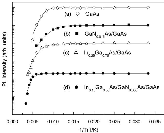
Fig. 4. Temperatures dependence of PL integral intensity for sample with (a) GaAs, (b) GaN<sub>0.016</sub>As<sub>0.984</sub> SCL, (c) In<sub>0.25</sub>Ga<sub>0.75</sub>As SRL, and (d) In<sub>0.15</sub>Ga<sub>0.85</sub>As/GaN<sub>0.008</sub>As<sub>0.992</sub>, respectively. The fitted curves are shown as solid lines.
