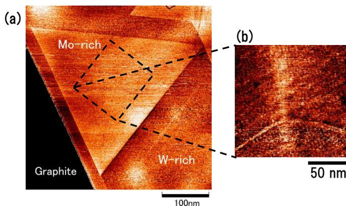
Fig.1 (a) Mo-rich area in Mo<sub>1-x</sub>W<sub>x</sub>S<sub>2</sub> monolayer
