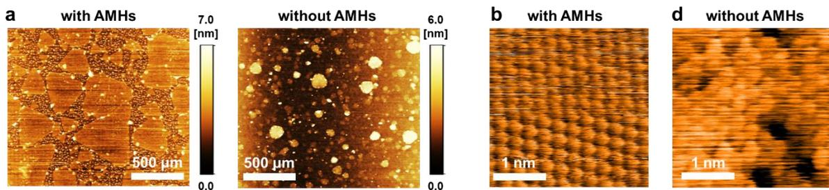
Fig.1 (a) AFM and (b) STM images of MoS<sub>2</sub> grown by MOCVD with and without alkali metal halide (AMHs).
