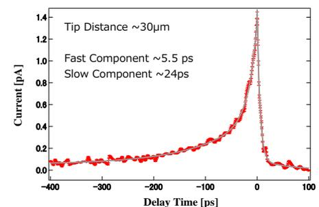
Fig. 2: Optical pump-probe spectrums obtained by laser focusing onto tip1 apex.
