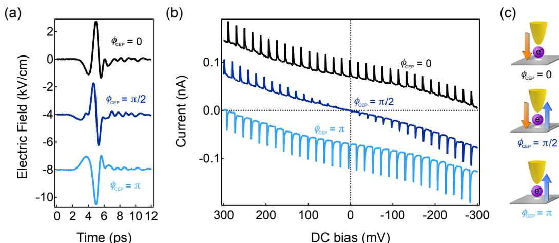
Fig. 2 (a) Waveforms of single-cycle THz electric fields with different CEPs ( $\phi_{\text{CEP}} = 0, \pi/2$  and  $\pi$ ) measured using EOS. (b) CEP dependence of tunnel current as a function of DC bias measured using a digital oscilloscope. The spectra with  $\phi_{\text{CEP}}=0$  and  $\pi$  are offset by  $\pm 0.07$  nA for clarity. (c) Schematics illustration of the electron tunneling processes through the junction. The orange and blue arrows show the tunneling direction.
