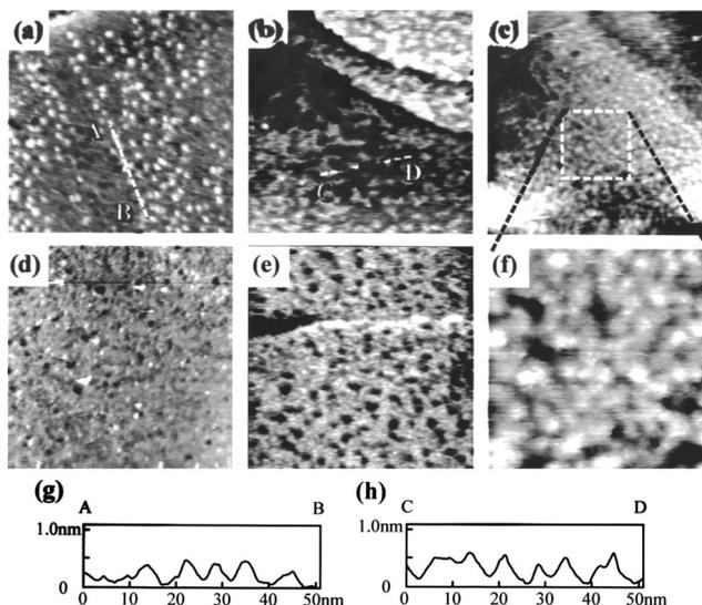
FIG. 2. STM images of  $\beta$ -CyD-SH on Au(111) formed by different immersion times (100 nm  $\times$  100 nm,  $V_s = 0.5$  V,  $I_t = 0.3$  nA): (a) 3 s, (b) 6 s, (c) 60 s, (d) 10 min and (e) 1 h, respectively, (f) magnification of (c). (g) and (h) cross sections along A–B in (a) and C–D in (b), respectively.
