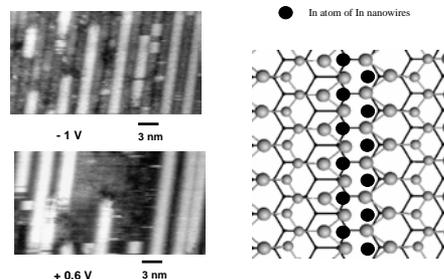
Nucleation and growth of In wires enhanced by step (Enrlich-Schwoebel) barrier
