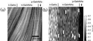
Fig.2 (a) STM image of a cleaved GaInNAs p-n junction interface.(b) SPV image obtained for the surface with Vs = +1.9V.
