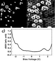
Fig. a) A STM image of  $C_{60}$ , b) the corresponding dI/dV image showing the distinct symmetries for the two different adsorption states, and c) the dI/dV curve for  $C_{60}$  on the glycine network.
