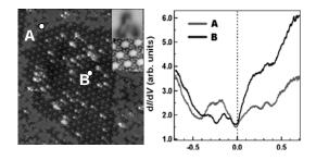
in the sample bias region from -400 mV to -100 mV Fig.1 STM image Fig.2 STS spectra shows that the original 2DEG on Cu(111) surface were changed by surrounding molecules. Details will be discussed at the colloquium.
