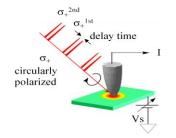
Fig.1 Schematic of time-resolved STM
