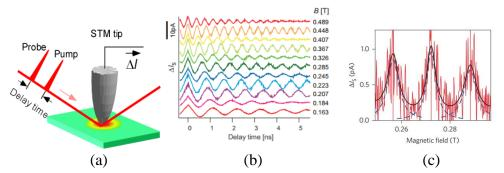
*Fig.1.* (a) The schematic of the OPP-STM. (b) The magnetic field dependence of spin precessions under the OPP-STM setup. (c) The resonant spin amplification result.
