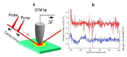
**Figure 1** (a) The basic schematic of OPP-STM experimental setup. (b) Sample: GaAs (110), red curve: the OPP-STM spectra of coherent phonon signal with sample bias voltage  $V_b$ =1.0V, tunneling current  $I_t$ =100pA; blue curve: the optical pump-probe reflectivity spectra of coherent phonon signal.
