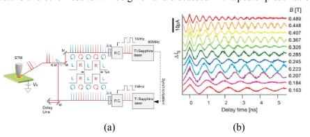
**Fig.1.** (a) The schematic of the OPP-STM. P.C is the pockels cell used to modulate the polarization states.(b) The magnetic field dependence of spin precessions under the OPP-STM setup, the spin precession occurs at the Larmor frequency  $\omega = g\mu_B B/\hbar$ , where g is the Landé's g factor, B is the magnetic field,  $\mu_B$  is Bohr magneton and  $\hbar$  is Dirac constant.
