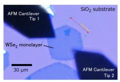
Fig. 1: Optical microscope image of the experimental setup.
