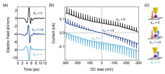
Fig. 2 (a) Waveforms of single-cycle THz electric fields with different CEPs ( $\phi_{CEP} = 0$ ,  $\pi/2$  and  $\pi$ ) measured using EOS. (b) CEP dependence of tunnel current as a function of DC bias measured using a digital oscilloscope. The spectra with  $\phi_{CEP} = 0$  and  $\pi$  are offset by  $\pm 0.07$  nA for clarity. (c) Schematics illustration of the electron tunneling processes through the junction. The orange and blue arrows show the tunneling direction.
