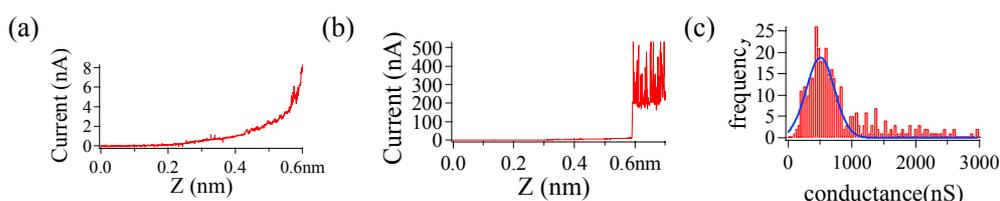
Fig. 3. I-Z curves obtained for (a) C8 and (b) 3TS2 molecules, respectively. (c) Histogram of conductance from the ohmic region ( $\pm 0.1V$ ) of I-V curves obtained for 3TS2 molecules.
