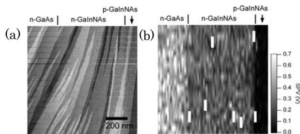
Fig.2 (a) STM image of a cleaved GaInNAs p-n junction interface.
