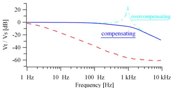
Fig. 1 . Bandwidth in potential measurement
