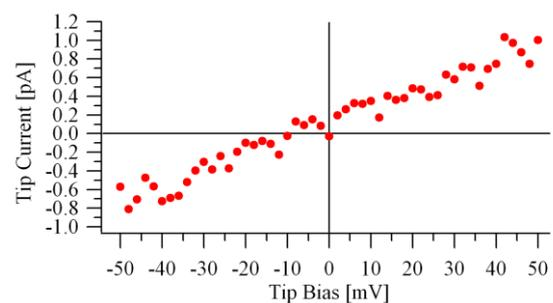
Fig. 2 . I-V characteristic of Au(111)
