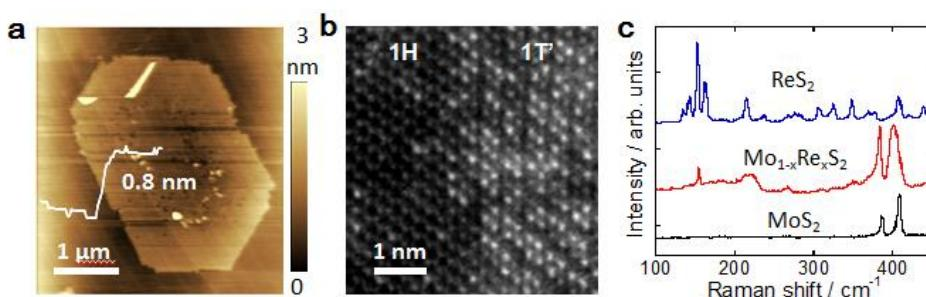
Fig.1 (a) AFM and (b) STEM images of Mo<sub>1-x</sub>Re<sub>x</sub>S<sub>2</sub>. (c) Raman spectra of MoS<sub>2</sub>, ReS<sub>2</sub>, and Mo<sub>1-x</sub>Re<sub>x</sub>S<sub>2</sub>.
