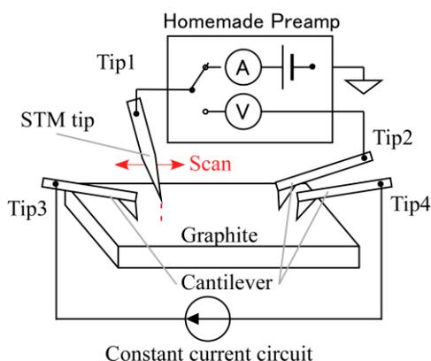
Fig. 1 Schematic of four-probe method
