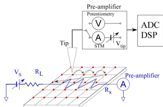
Fig. 2 Measurement concept of STM and STP
