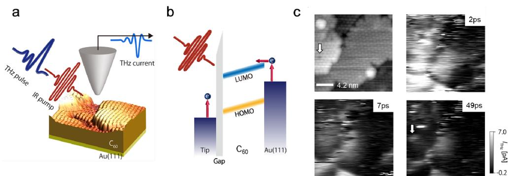
Figure. a. Illustration of experimental setup b. band diagram of STM tunneling junction under pulse excitation c. STM image of  $\text{C}_{60}/\text{Au}(111)$  surface and corresponding  $I_{\text{THz}}$  map taken with fixed delay time (2 ps, 7 ps, 49 ps)
