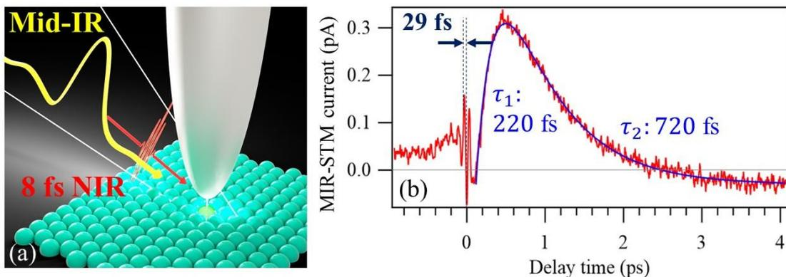
Fig. 1, (a) Schematic of 8 fs NIR-pump MIR-STM. (b) Ultrafast modulation of tunneling current in a tunnel junction of MoTe<sub>2</sub> and Pt/Ir tip. The pump pulses were incident at delay time = 0 ps.
