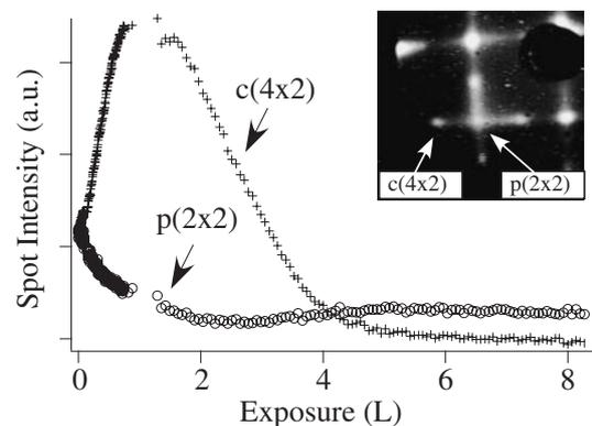
Fig. 2. LEED spot intensities for the  $(-1/2, -1/2)$  and  $(-3/4, -1/2)$  spots as a function of the Kr gas adsorption (30 V, 25 K). The change at  $\sim 1.6$  L is just due to the measurement procedure.
