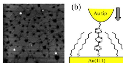
Fig. 1. (a) STM image of isolated 3TS2 molecules (bright spots) embedded in a C8 film (75nm×75nm). (b) Schematic of the “point contact method” by STM.
