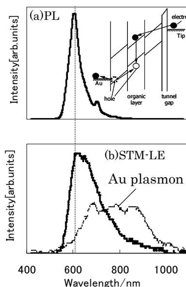
**Fig.1** (a) A PL spectrum from rubrene powder (**Inset:** Energy diagram of the layer structure); (b) A sequential STM-LE spectra from Alq<sub>3</sub>/rubrene/TPD/Au obtained in air at room temperature (Bias voltage: 5.0 V, tunneling current: 3 nA, exposure time of CCD: 128 sec/spectrum). Thick and thin lines stand for first and second measurements.
