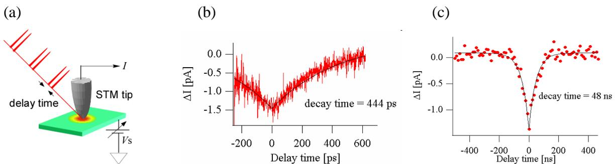
Fig. 1. (a) Schematic of PPX-STM. PPX-STM spectra obtained for (b) low-temperature grown GaNAs and (c) n-type GaAs ( $10^{18} \text{ cm}^{-3}$ ).
