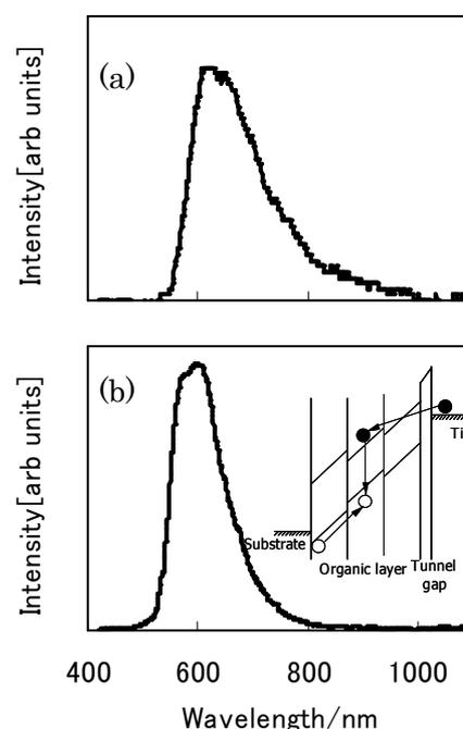
**Fig.1** (a) A STM-LE spectrum from Alq<sub>3</sub>/rubrene/TPD/Au obtained in air at room temperature (Bias voltage: 5.0 V, tunneling current: 3 nA, exposure time of CCD: 128 sec/spectrum). (b) A STM-LE spectrum from Alq<sub>3</sub>/rubrene/TPD/ITO obtained in air at room temperature. (Bias voltage: 6.0 V, tunneling current: 5 nA, exposure time of CCD: 128 sec/spectrum). (**Inset:** Energy diagram of the layer structure)
