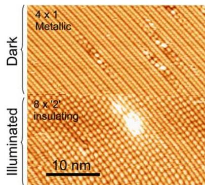
Fig. 1. Optical control of metal (upper area) to insulator (lower area) transition.
