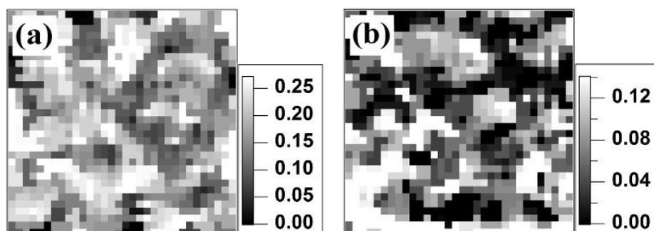
**Fig. 1.** 2D mapping of light emission intensity from (a) Alq<sub>3</sub> ( $\lambda=530\pm 20$  nm), and (b) Rubrene molecules ( $\lambda=600\pm 30$  nm), respectively. (scan width:  $1000\times 1000$  nm<sup>2</sup>)
