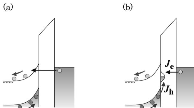
Fig. 4 1-D energy band diagram of tunnel junction
