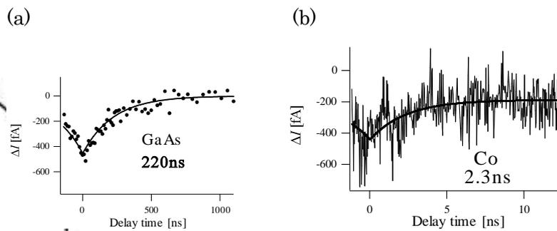
Fig. 3  $\Delta I$  vs. delay-time curve obtained above (a) bare GaAs (b) Co/GaAs
