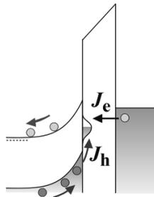
Fig.2: Schematic of recombination mechanism via gap states.
