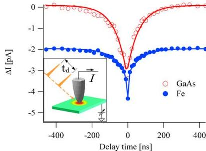
Fig.1:  $\Delta I$  vs delay time obtained above a bare GaAs surface and a Fe nanoparticle
