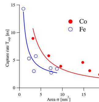
Fig.3: Lifetime (capture time) of holes via gap states as a function of nanoparticle size.
