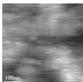
Fig. 1 STM image obtained for  $V_t=4.0V$  and  $I_s=150pA$ .
