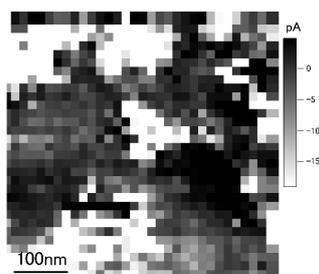
Fig. 2 Dark current mapping for  $V_s = -3.7V$ .
