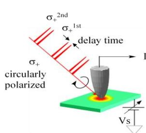
Fig.1 Schematic of time-resolved STM
