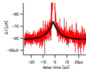
Fig.2 TR-STM spectra obtained for an undoped GaAs. Peak at 0 delay is due to interference between laser pulses.
