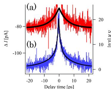
Fig.2 (a) TR-STM and (b) OPPR spectra obtained for an undoped GaAs.
