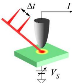
Fig.1 Schematic of time-resolved STM
