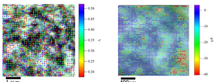
Figure 2: Voc distribution measured by Light-Modulated STM.
