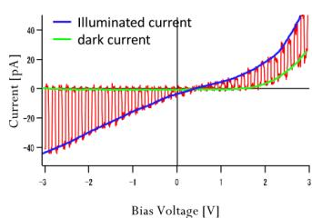
Figure 1: Typical Light-Modulated I-V spectrum.
