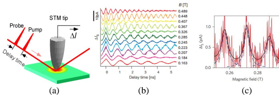
**Fig.1.** (a) The schematic of the OPP-STM. (b) The magnetic field dependence of spin precessions under the OPP-STM setup. (c) The resonant spin amplification result.
