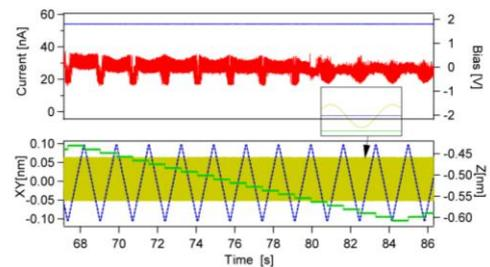
Fig.2 Tunneling current measured with 3D change in the STM tip positions (upper graph, red: current, blue: bias voltage, and lower graph, blue: x, green: y, yellow: z positions).
