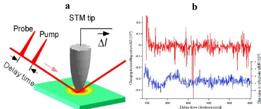
**Figure 1** (a) The basic schematic of OPP-STM experimental setup. (b) Sample: GaAs (110), red curve: the OPP-STM spectra of coherent phonon signal with sample bias voltage  $V_b=1.0$ V, tunneling current  $I_t=100$ pA; blue curve: the optical pump-probe reflectivity spectra of coherent phonon signal.
