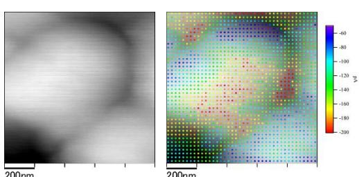
**Fig. 1:** STM topography obtained for  $V_t = 2.0$  V,  $I_s = 30$  pA (left) and photocurrent mapping for  $V = -2.7$  V (right).
