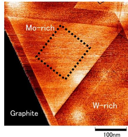
Fig.1 STM image of  $\text{Mo}_{1-x}\text{W}_x\text{S}_2$  Island
